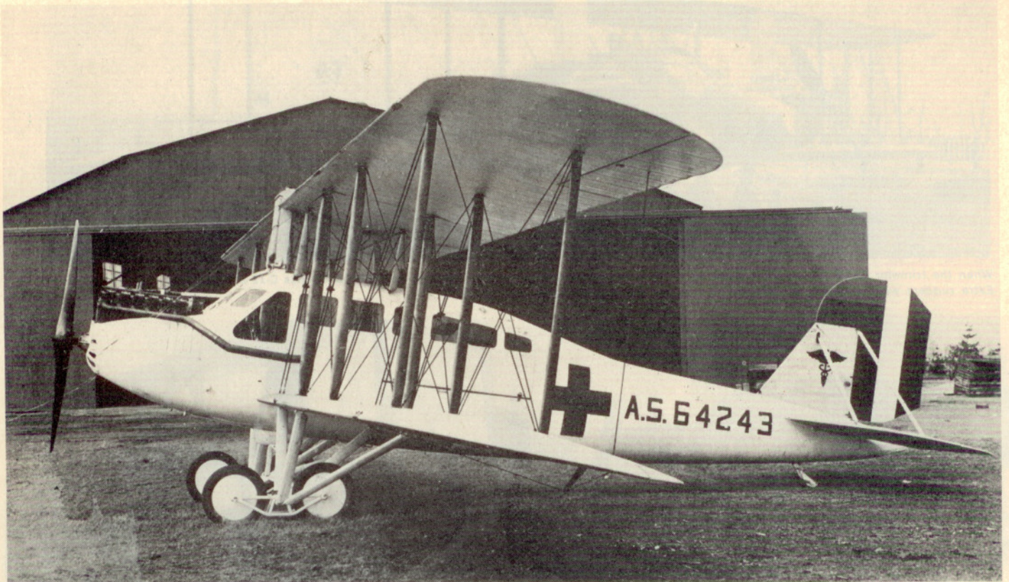
The only customer to buy more than one Eagle was the U.S. Army, which bought three single-engine versions powered with the 400-hp Liberty. This one has been converted to an aerial ambulance, complete with red crosses and all-white coloring.
